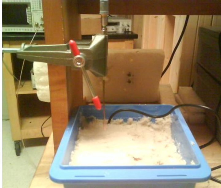
Figure 2.3 Probe inserted in the sand for good contact
